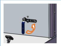
7. During the sweeping process, when there is more dust on the ground and it is necessary to turn on the sprinkler function, rotate the sprinkler valve from the vertical position to the horizontal position as shown in the figure.
